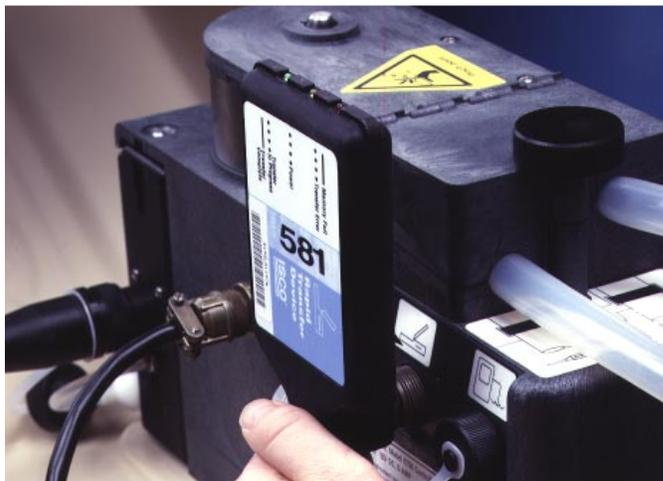
The Isco 581 RTD provides a fast, simple way to collect and transport data from 6700 Series Samplers.
